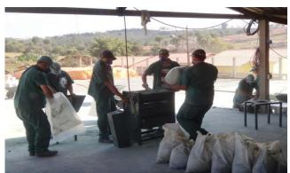
Figure 11.2.2-5 Riffle Splitting RC Samples
