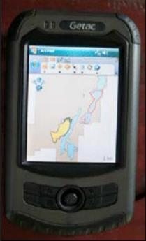
Figure 9.1.1-2 Geological Mapping using GETAC PDA's with ArcPad Software (VERDE, March 31, 2013)
