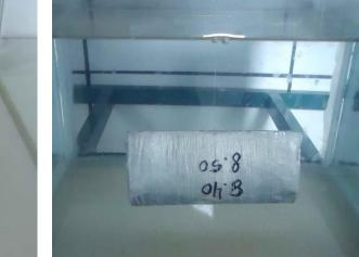
Figure 10.10-1 Wrapped Sample Weighed in Air
